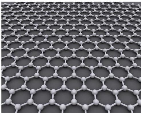
The ideal crystalline structure of graphene
