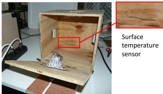
Different groups of students can be supplied with different house models having the same dimensions and constructed using different materials. The heater and the sensor are placed as reported **previously**.
