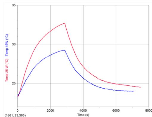
2. Heating and cooling curves of house models constructed with plasterboard core vs. polystyrene core:
